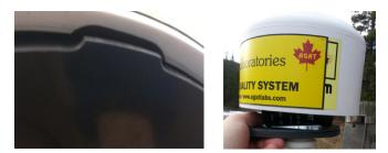
**8.** Lift upwards, keeping the passive holder level, until the horizontal grooves at the top of the vertical grooves are visible.
