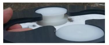
**6.** Carefully gripping the sides of the pucks, one-by-one lift them clear of circular seats and set on clean, level area, sampling surface side facing upwards.
